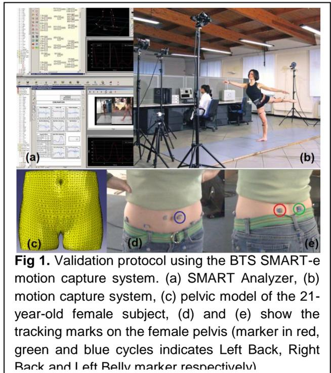
**Fig 1.** Validation protocol using the BTS SMART-e motion capture system. (a) SMART Analyzer, (b) motion capture system, (c) pelvic model of the 21-year-old female subject, (d) and (e) show the tracking marks on the female pelvis (marker in red, green and blue cycles indicates Left Back, Right Back and Left Belly marker respectively)
