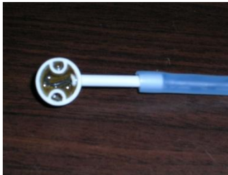
Figure 2: Redesigned electrode currently undergoing evaluation. The stainless steel electrodes are now housed such that they are approximately 1mm from the electrode surface. Conductive paste is injected into the recessed cavities that house the electrodes. Suction is still used to hold the electrode in place on the vaginal wall.
