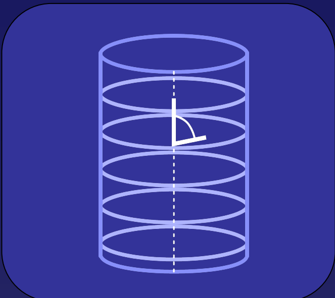
b)Contracting fibers at angles greater than 55 resist circumferential expansion
