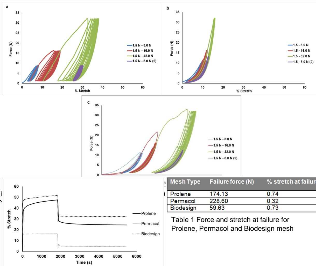
Figure 2 Stretch vs. time for Prolene, Permacol and Biodesign mesh samples
