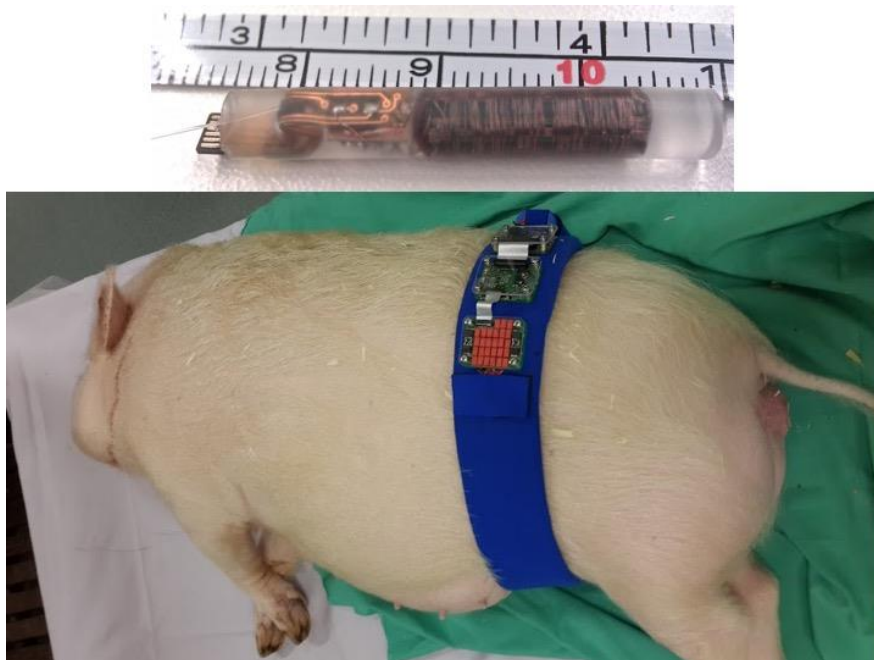
Fig 1. Bladder Pill (top, scale cm) and animal fitted with band containing coil, receiving circuit and battery (bottom)
