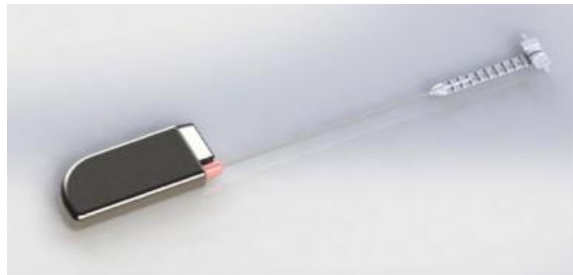
Fig 1: View of the Artificial Sphincter. The motor pulls on the cuff to modulate its diameter. The cuff is closed around the urethra.
