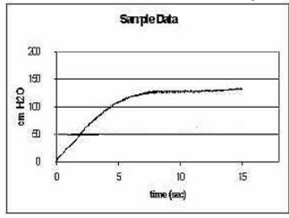
Bench testing was performed to assess the URP waveform and to evaluate the reproducibility of the URP measurement using an adjustable NIST certified pressure gage (artificial sphincter) to test seven prototype units.
