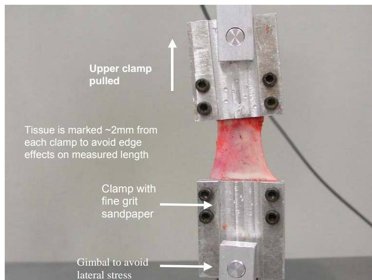
**Figure 2. Sample Tensile Testing Configuration**
