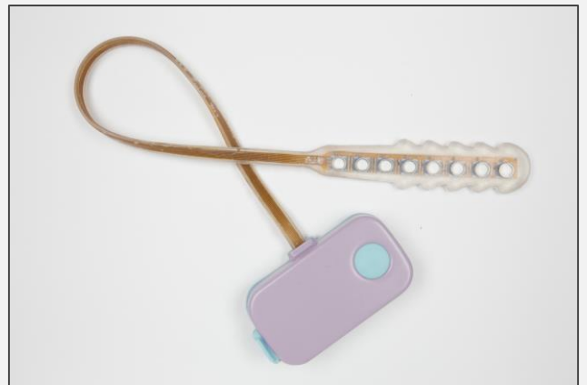
The FemFit® utilises a linear array of eight pressure sensors to distinguish between intra-abdominal pressure and pelvic floor pressure within the vaginal pressure profile.
