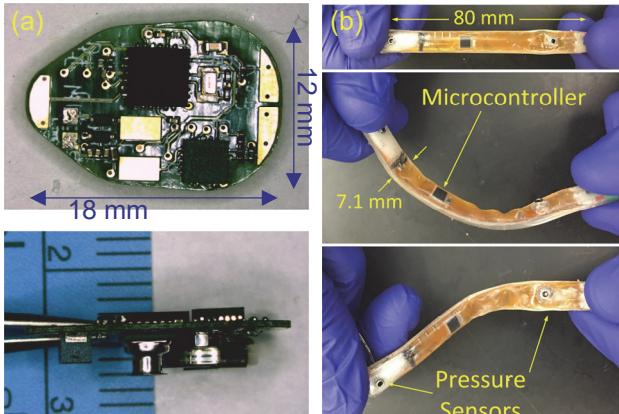
Wireless bladder sensor (a) designed for suprapubic insertion into a feline bladder. The bowel sensor (b) was longer with a flexible form factor that is more appropriate for porcine models.
