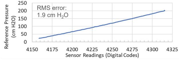
Pressure sensor calibration curve with linear response and 1.9 cm H<sub>2</sub>O root mean square error.
