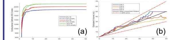
Volume sensor variation with feline urine concentration (a) was partly corrected with a concentration sensor (b). Low overall volume accuracy was sufficient to estimate bladder state (e.g. bladder half full vs bladder empty).
