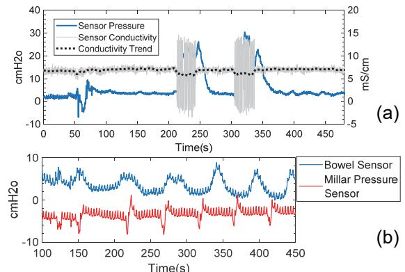
Bowel sensor detected contractions evoked by stimulation in proximal colon (a) and local phasic contractions in transverse colon separately from a distal manometry catheter (b). Data from anesthetized adult male Yucatan pig. Data generated in collaboration with Drs Larauche and Million et al. (SPARC, UCLA).
