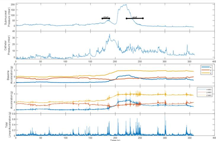
**Figure 2.** Data from a single voiding episode. Acceleration is separated at a cut-off frequency of 0.15 Hz into gravity component and linear acceleration. Magnitude of total linear acceleration is calculated by the following formula
