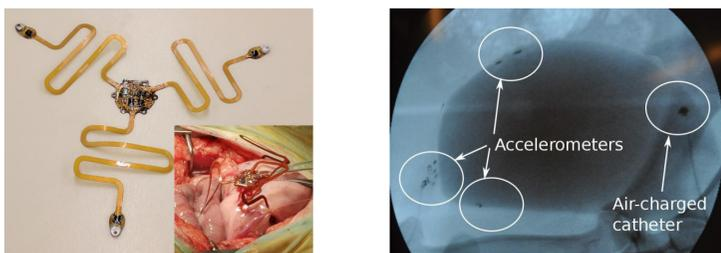
**Figure 1.** Acceleration measurement device, sensors are placed on three satellite arms and one on the central island.
