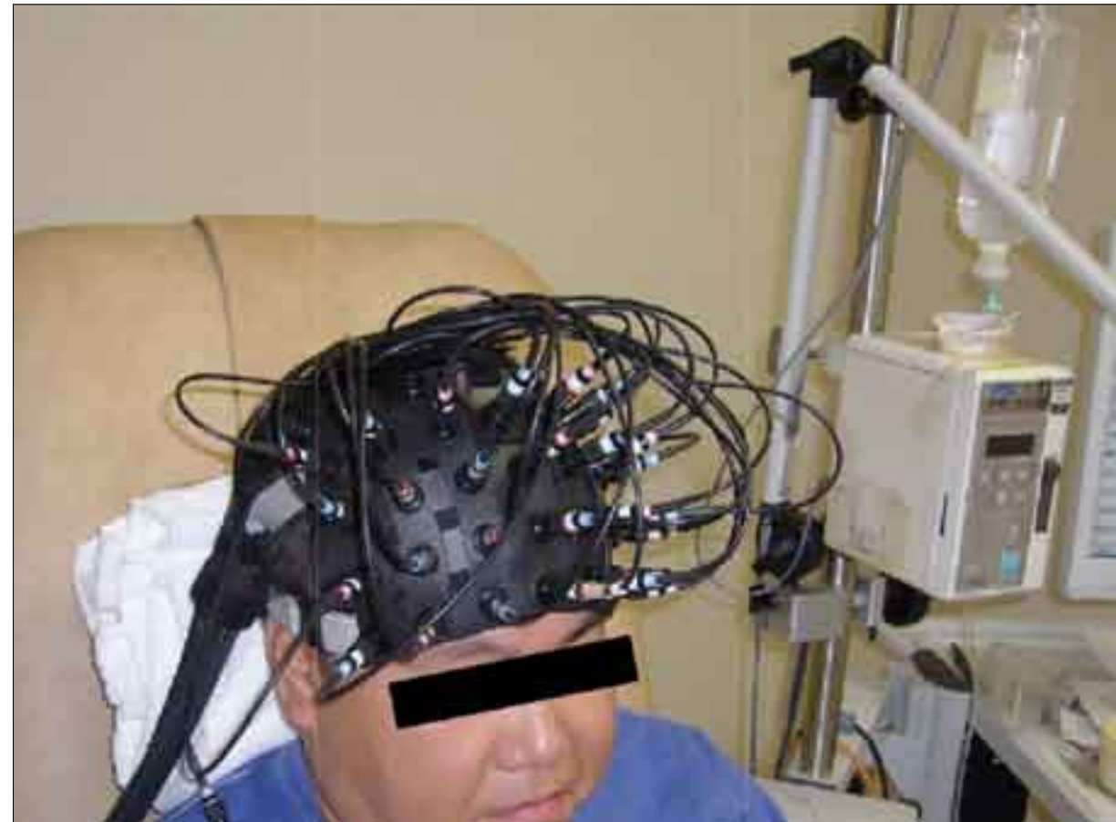
Fig. 1: Head gear with the probe array for fNIRS. Upper panel: The head gear is small and light (hundreds of grams). Lower panel: The head gear is equipped with 16 light emitting and 17 detector probes, and 52 channels can be measured simultaneously.
