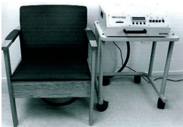
Figure 6 : Magnetic stimulation chair with external power unit (Courtesy of Professor Kate Moore and Dr Alastair Morris, University of Sydney, Australia)
