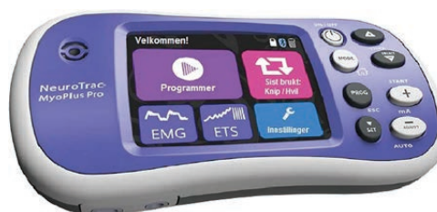
FIG. 7 Verity Medical NeuroTrac MyoPlus Pro surface electromyography biofeedback apparatus (also incorporating electrical stimulation (reproduced with permission from Quintet, Norway)
