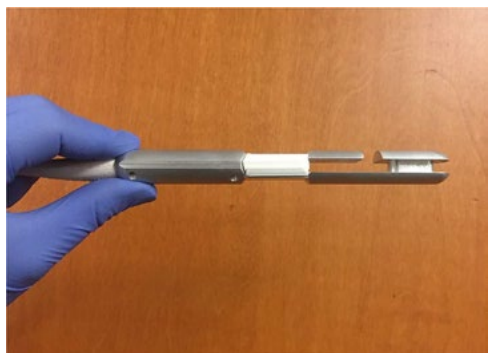
FIG. 5 Ann Arbor, USA, dynamometer speculum. Note that the bills of the speculum are covered by a condom when in use (reproduced with permission from J.A. Ashton-Miller, R. Zielinski, J.O. DeLancey, J.M. Miller)
