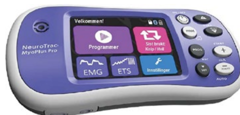
FIG. 7 Verity Medical NeuroTrac MyoPlus Pro surface electromyography biofeedback apparatus (also incorporating electrical stimulation (reproduced with permission from Quintet, Norway)
