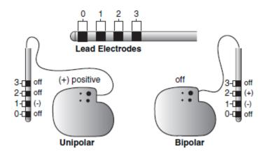
The four electrodes on a lead can be configured with or without the neurostimulator case in the following two configurations:
